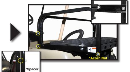
Attach bottom of Armrests to Footrest using the Footrest Brackets and 10x70mm bolts from Pack 3.
